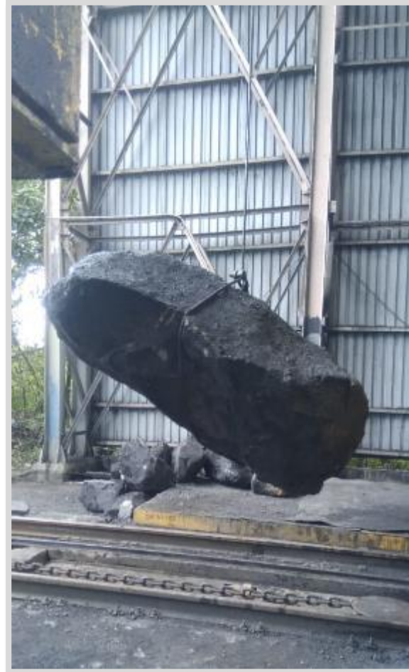
Coal Boulder lifting
